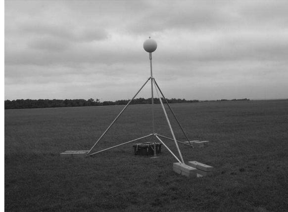
Figure 1: Photograph from September 2003 showing the ET probe deployed in Beaufort, NC for Hurricane Isabel. The white ET sphere is mounted on an aluminum tripod.
