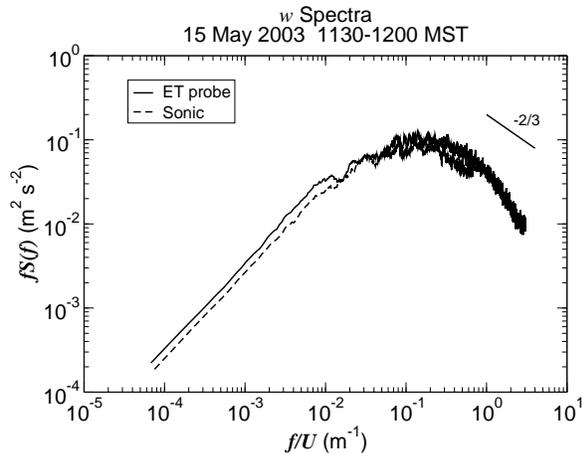
Figure 2: Comparison of ET probe and sonic anemometer power spectra for the vertical velocity component.  $f$  is the frequency,  $S(f)$  is the spectrum, and  $U$  is the mean wind speed.
